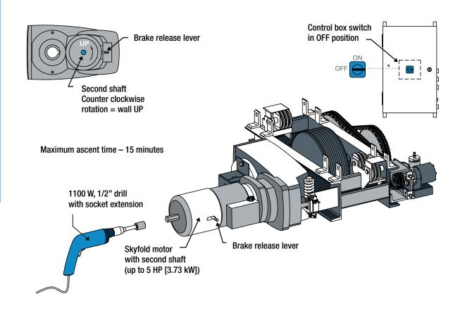
In the unlikely event that the Skyfold wall does not respond to the key switch operation, it can now be operated by using a heavy duty drill. A shaft extension has been added to the motor allowing for an alternative method of raising and lowering the wall. This feature is now standard on all of our walls. This diagram is for illustration purposes only. Please refer to the applicable operating procedures for complete instructions.
